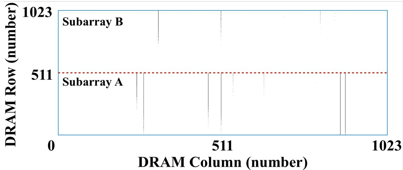
Figure 4: Activation failure bitmap in  $1024 \times 1024$  cell array.
