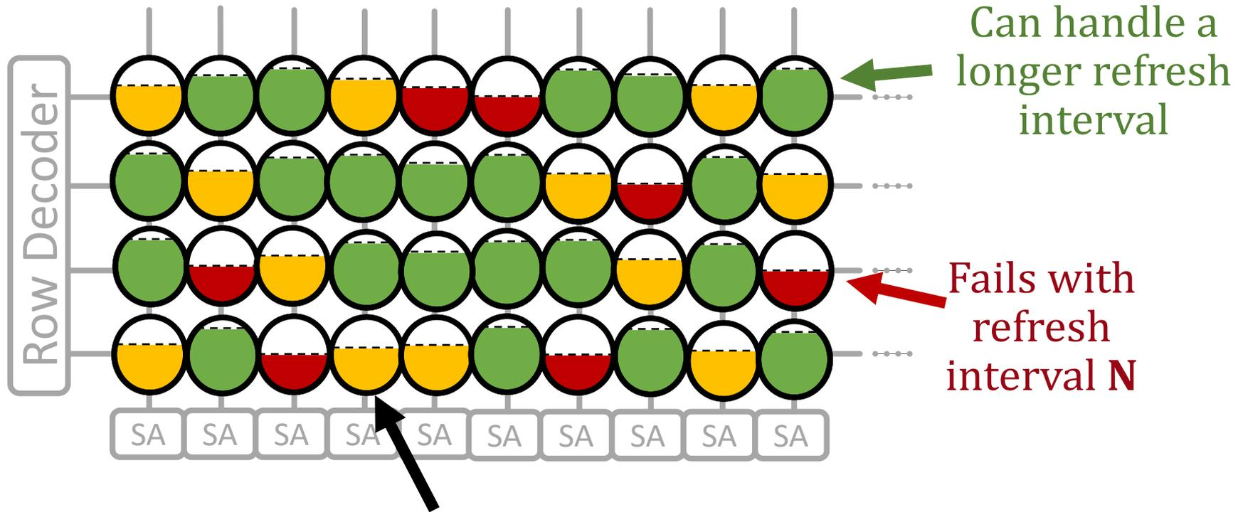
After time  $N$ , some cells leak close to  $V_{min}$ .
