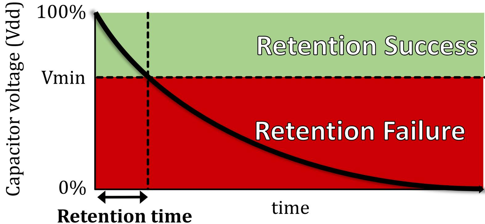
**Retention failure** – when leakage corrupts stored data
