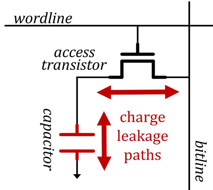
Stored data is **corrupted** if too much charge leaks (i.e., the capacitor voltage degrades too much)
