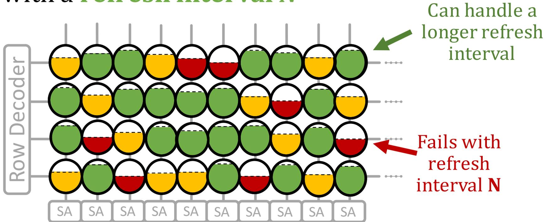
The pattern of retention failures across a segment of DRAM is **unique** to the device
